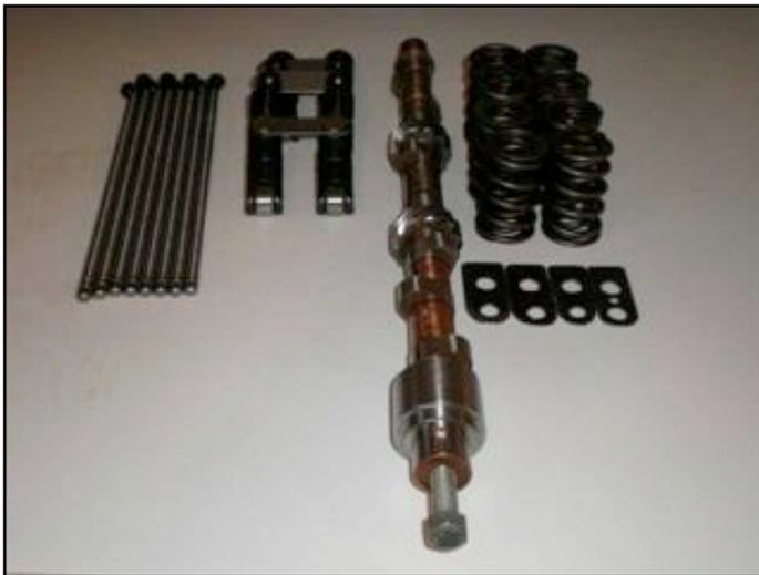
From a performance standpoint, roller cams offer a tremendous advantage over flat lifter cams. A roller lifter can handle a much steeper ramp on a cam lobe than a flat bottom lifter. This allows roller cams to open the valves more quickly so they can reach maximum lift earlier in the timing cycle. When you plot valve lift and duration on a graph,
